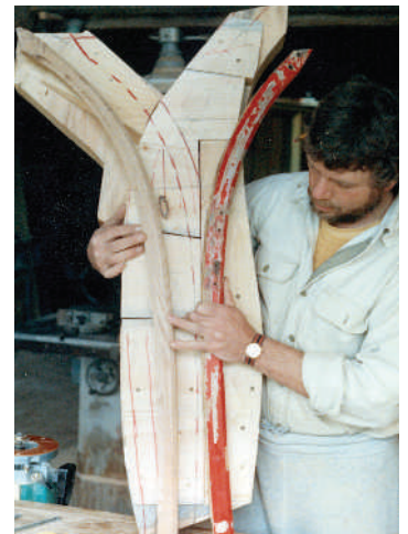
Chance Anderson Recreating parts—the red piece is from the old coach. The form was created based on that piece. The form helps generate both right and left pieces. The pieces themselves are cut from the solid so the form is more of a pattern to cut and shape to rather than to bend on.
