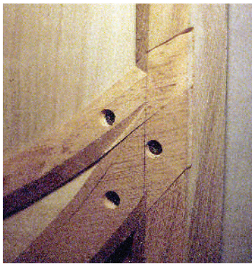
Intersection of quarter panel(s) framing with corner post. The use of wood screws was commonly used as a holding technique and we continued this tradition.
